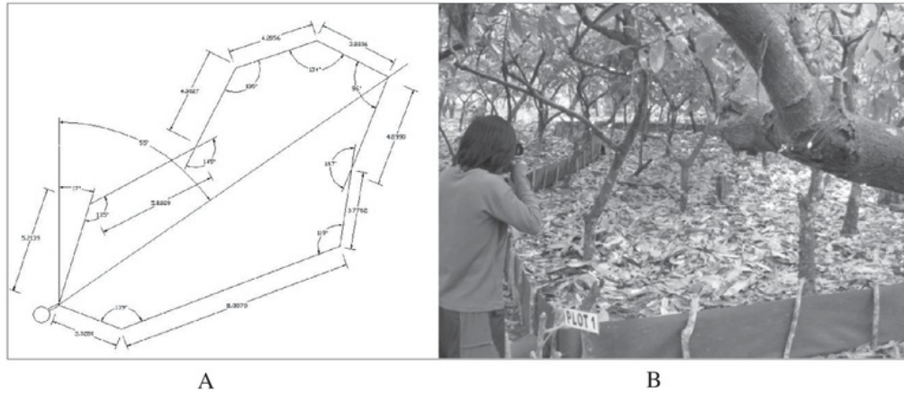
Fig. 1. Experiment plot used to measure water run off and erosion. Lay out of the experiment plot (A) and experiment plot (B).
